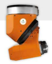
Two axis head with fork structure, optimized for mold and die machining on 5-axis machine tools; integrates modules with Technai Direct Drive motors on both axis, and is available with electrospindles up to 24.000 rpm and 50 kW, HSK-A63 or HSK-A100 tool holder. TCH 19 head is designed to equip big machines for mold and die machining, particularly suitable for plastic-injection mold and die in which the slim and penetrating electro spindle body structure suits the application at best.
