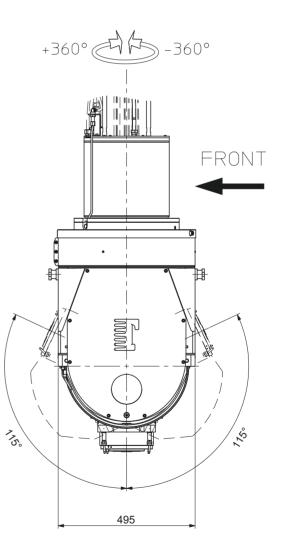
Two axis head with fork structure optimized for heavy 5-axes machines, integrates modules with Technai Direct Drive motors on both axes, and is available with electrospindles up to 12.000 rpm and 40 kW, HSK-A100 tool holder.
